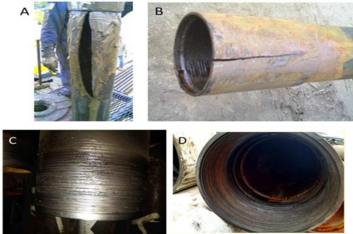
FIGURE III.9. MANUFACTURING DEFECT-INDUCED CASING FAILURE
