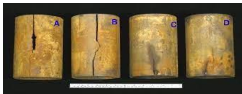
FIGURE III.8. MECHANICAL DAMAGE-INDUCED CASING FAILURE
