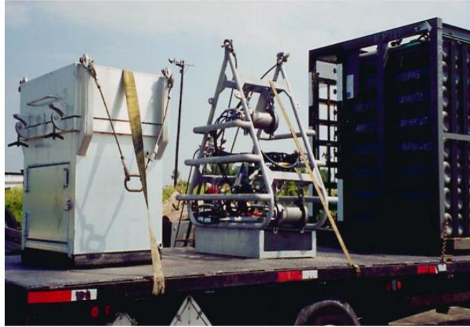
Figure II.8. High-pressure source to generate the airgun [17]
