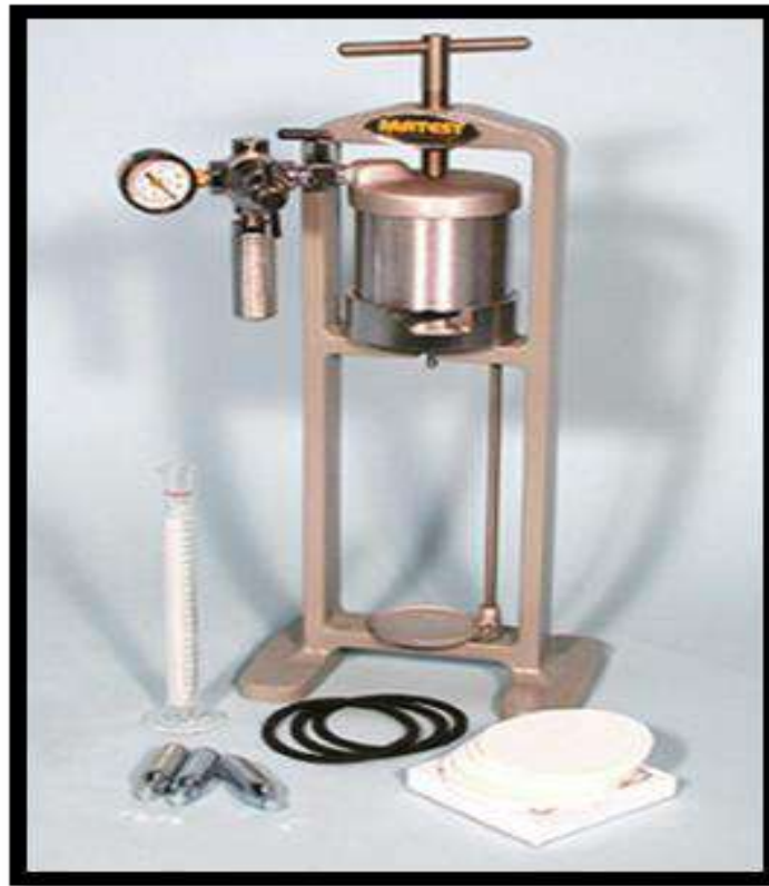
Figure I-07: l'appareil API filter press / LPLT filter press.
