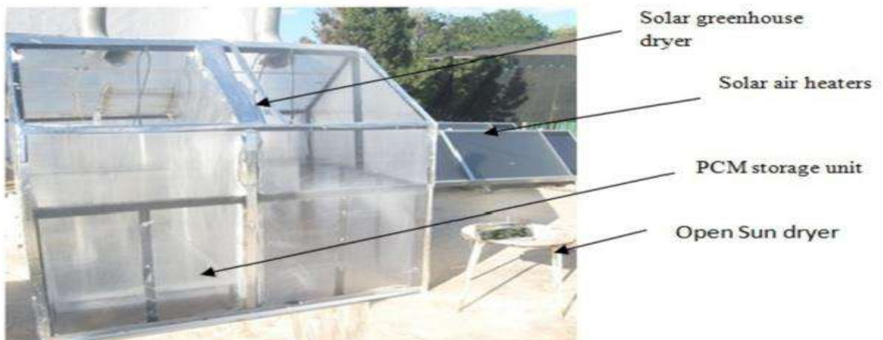
Figure II.10 Experimental solar greenhouse drying system. [36]
