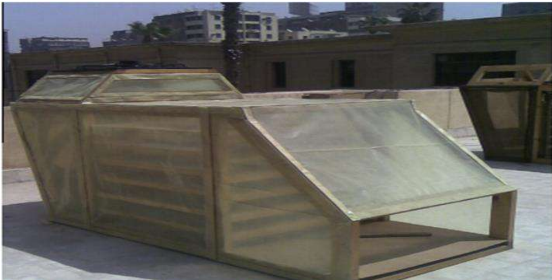
Figure II.7 Photograph of the direct solar dryer. [34]
