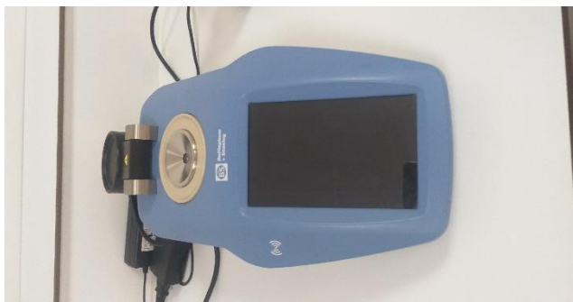
FigureII.10: Bellingham+ Stanely RFM300-M Refractometer
