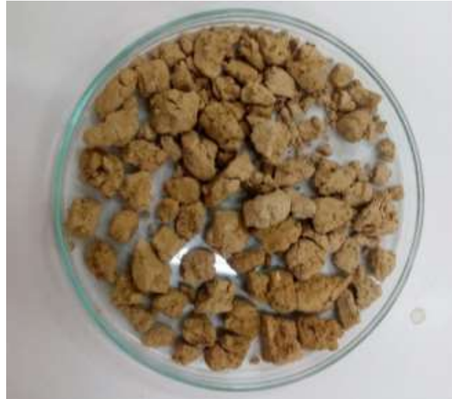
Fig.III.28: Cutting Saturation with \text{CaCl}_2 .
