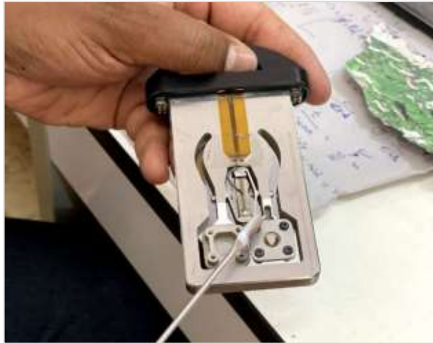
Fig.III.13 : Core Holder with Well A Core Samples for XRD Analysis.
