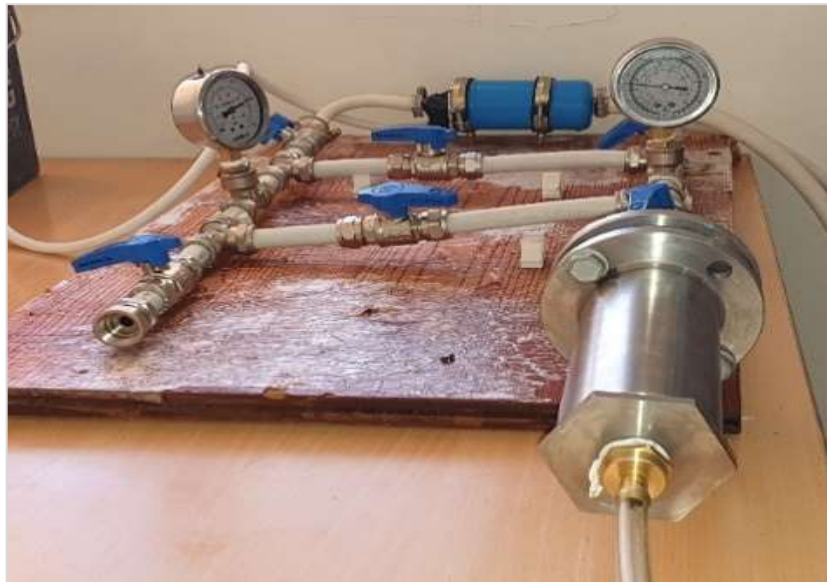
Fig.III.27: Installation schematic of the permeability measurement of reservoirs samples.
