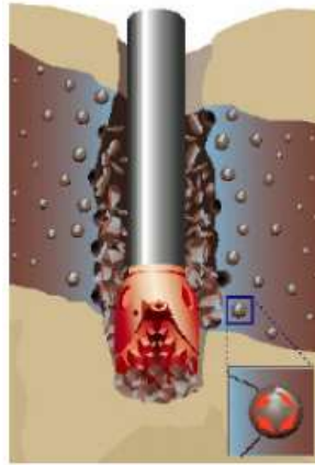
Fig.II.2: Naturally over-pressured shale collapse [46].
