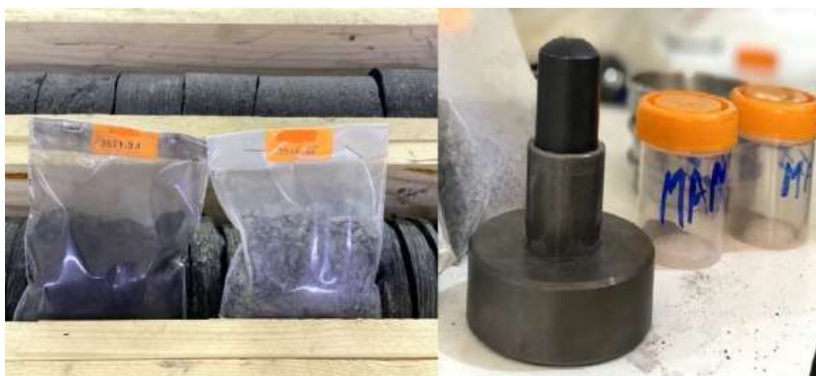
Fig.III.12: Core Samples from Wells A and B for XRD Analysis.
