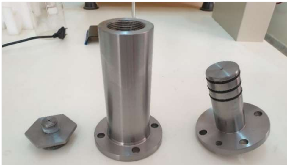
Fig.III.20: Piston components of the installation (Plug, cylinder, piston) [64].
