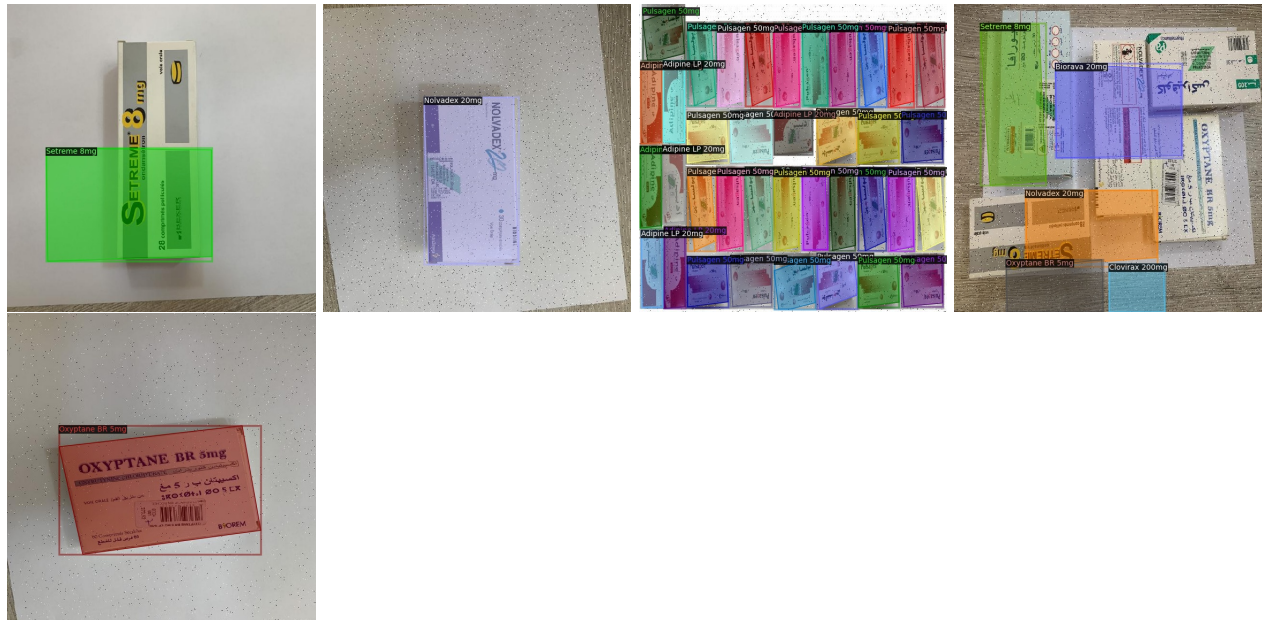
Figure 5.8: Result of Faster RCNN
