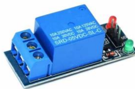
Figure 9: relai 5v de la carte 'Sensor'[12]
