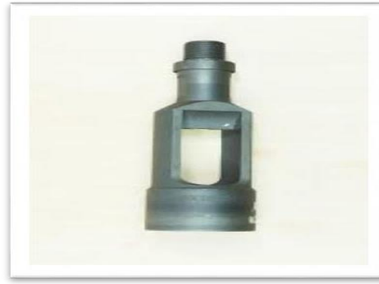
Figure III.1: Gauge Cutter (outil wire line).
