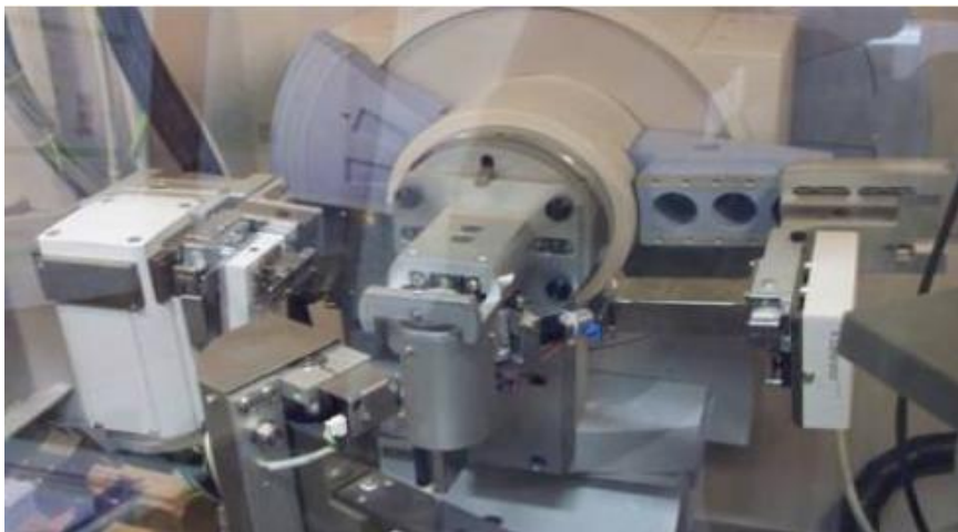
Figure III.5 : Diffractomètre Panalytical X'Pert Pro de type Bragg-Brentano.
