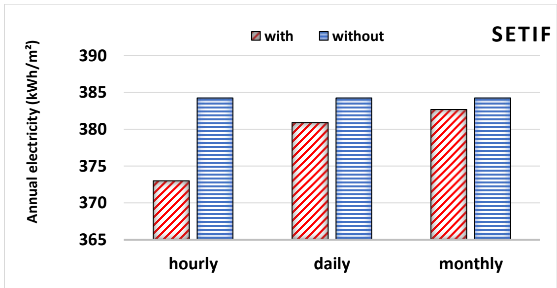
Figure 3.4: Annual estimated electricity with and without and without temperature effect in Setif
