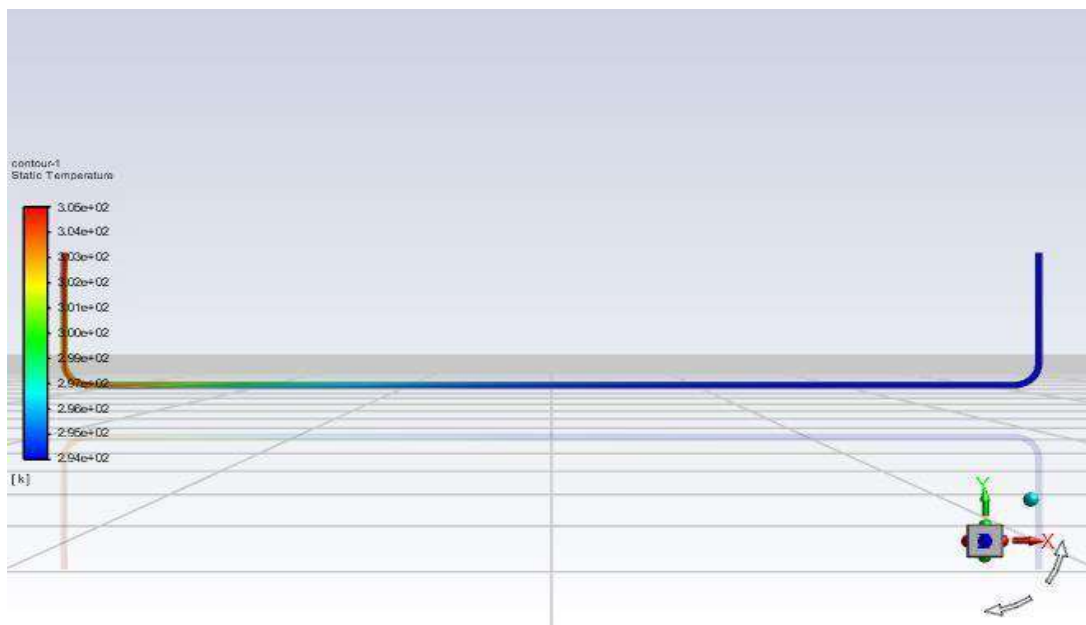
Figure III-15: The evolution of the air temperature in the tube - Re = 1500 with an adiabatic sort
