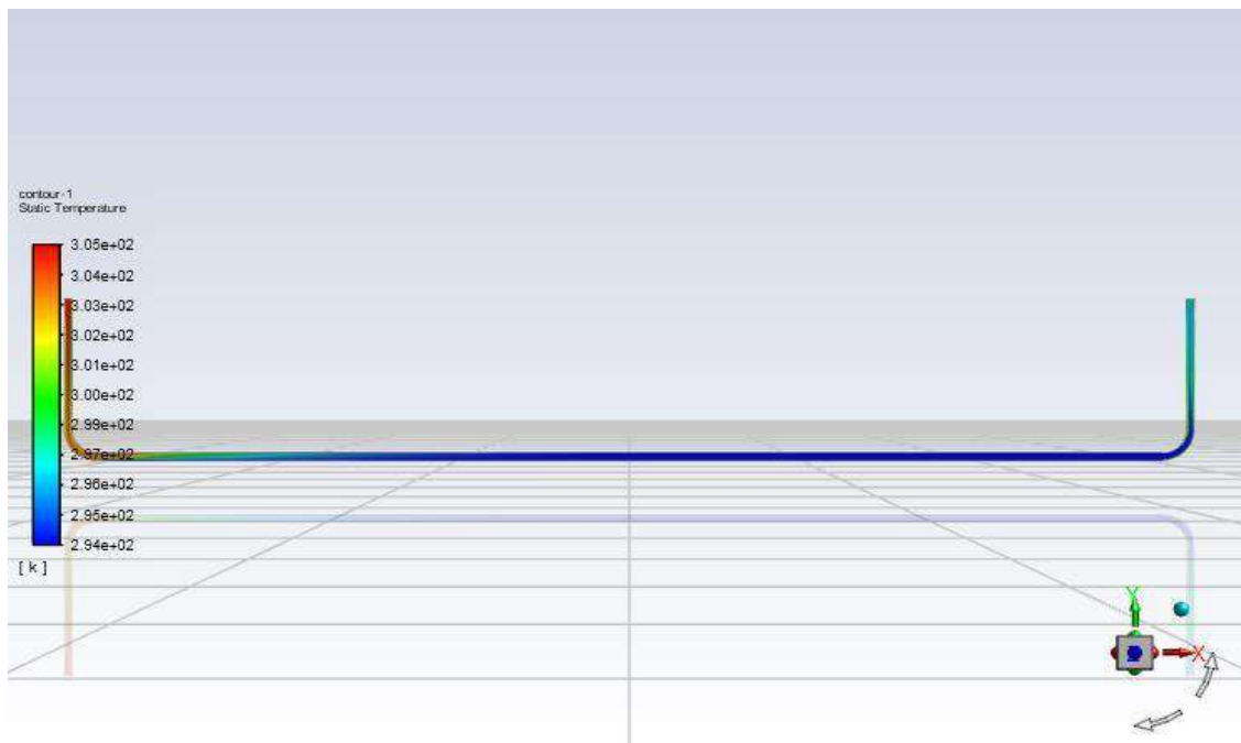
Figure III-13 The evolution of the air temperature in the tube – Re = 1000 with an normal sort
