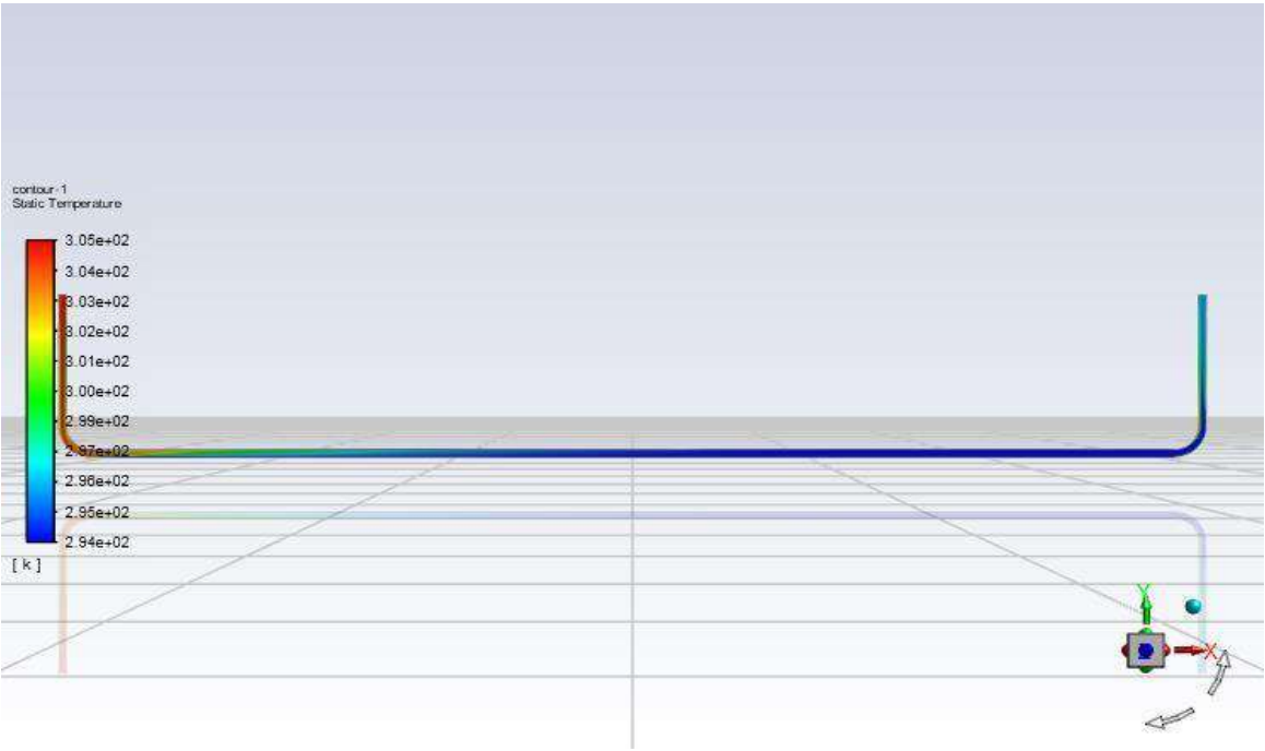
Figure III-17: The evolution of the air temperature in the tube - Re = 1500 with an normal sort
