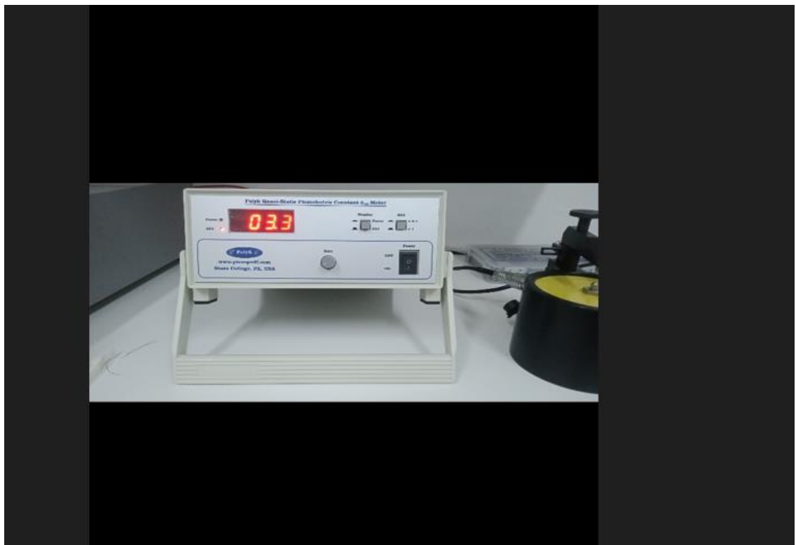
Figure III.5 : Piezometer d_{33} device
