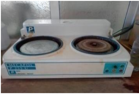
Figure II.4: The mechanical polishing device used to clean the sample
