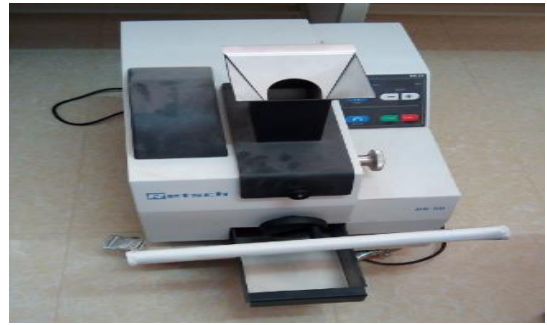
Figure II.5: The mechanical grinding device used to crush the sample
