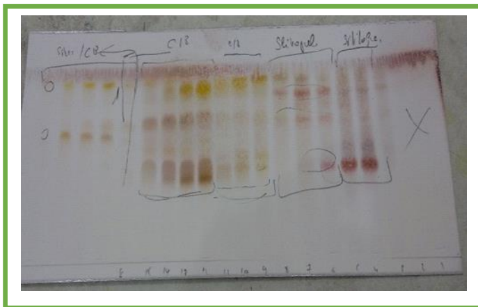
Figure 18: TLC of the first column fractions after collection of similar ones after the revelation
