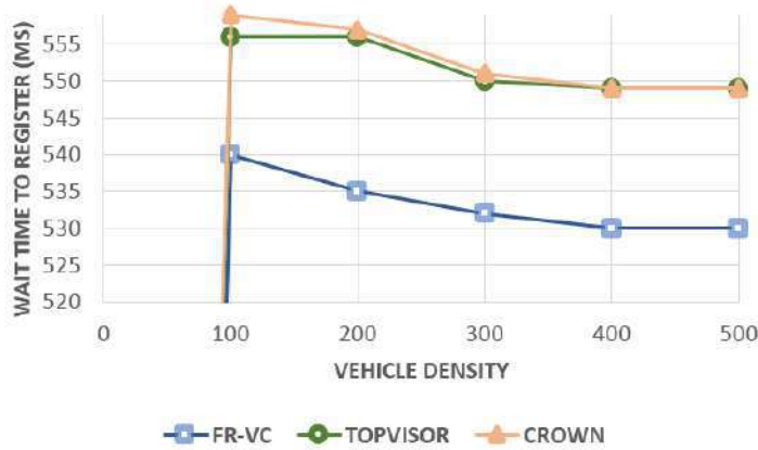
Figure 19. Performance evaluation comparisons of FR-VC with CROWN and TOPVISOR in terms of W_time.
