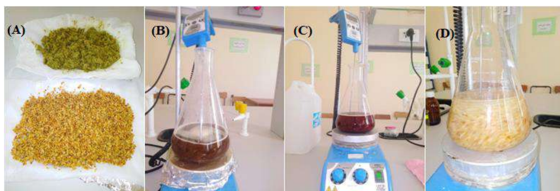
Figure III. 3: A photos showing the different stages of cellulose extraction (A: Washing, B: acid treatment, C: basic treatment, and D: bleashing)
