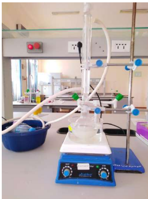
Figure III. 4: A photo showing the assembly of synthesis of cellulose nanocrystals (CNCs)
