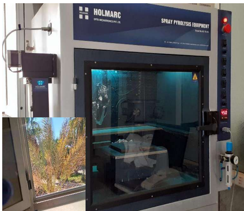
Figure III.1: Spray pyrolysis equipment used in LRPPS laboratory (Inset shows the obtained pure ZnO film).
