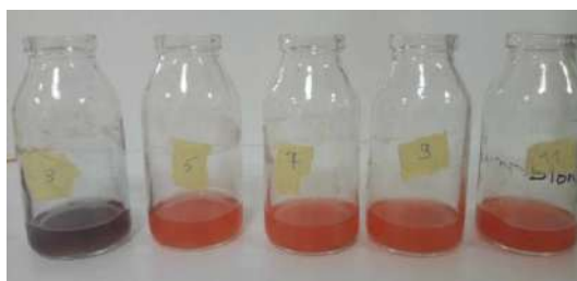
Figure.III.16: Photocatalytic degradation of Congo red under visible light irradiation using \text{NH}_3[\text{Cd}(\text{C}_2\text{O}_4)_2] \cdot 2\text{H}_2\text{O}
