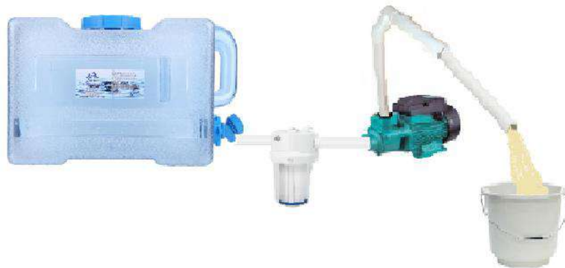
Figure VII.4: Experimental setup used in clay purification.
