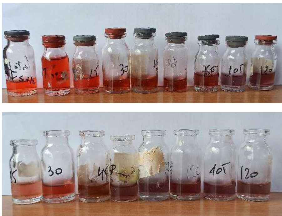
Figure.V.12: photos of adsorption reactions of FS1/2 and FS5.
