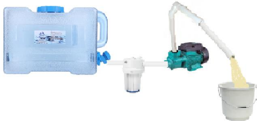
Figure VII.4: Experimental setup used in clay purification.
