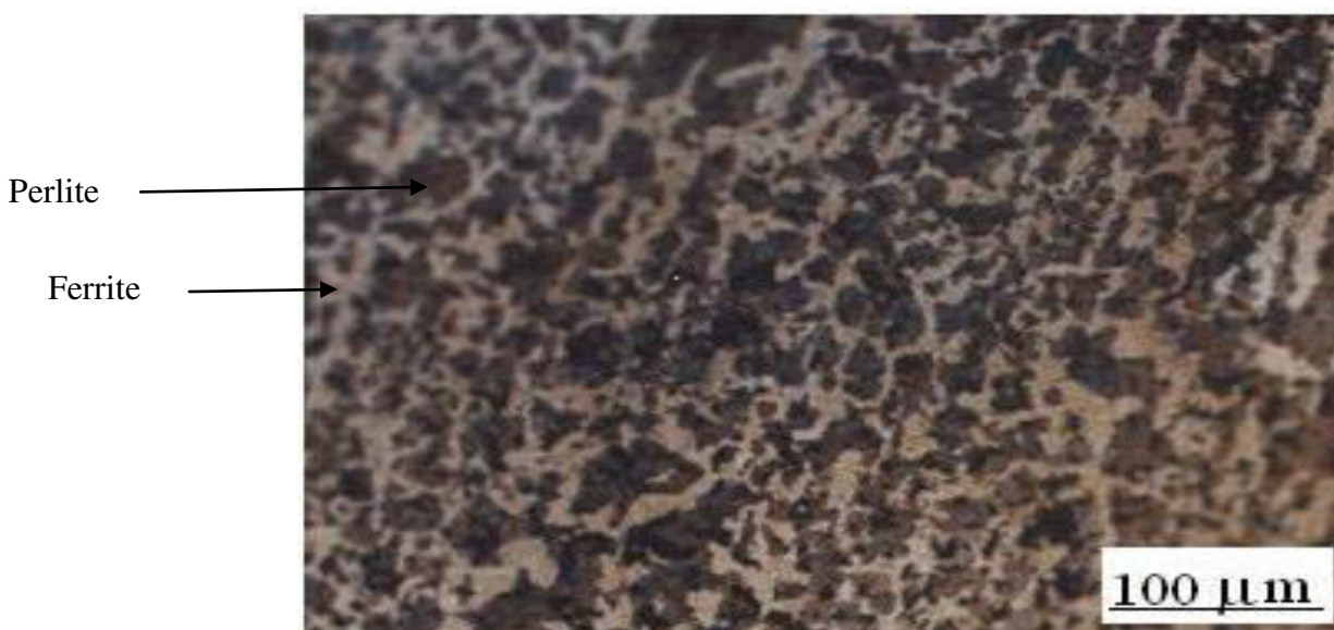
Figure II.3: Microstructure de l'AISI 1060 [72].
