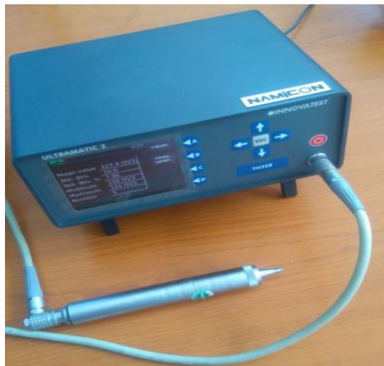
Figure II.5 Hardness Tester Ultramatic 2 HV400.
