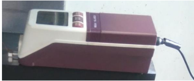
Figure II.4 Mitutoyo Surftest SJ-201 roughness meter.
