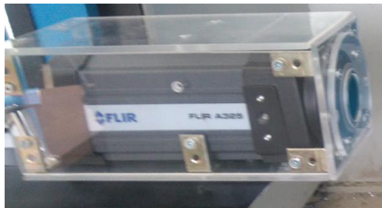
Figure II.3 Flir A325 infrared thermal camera.
