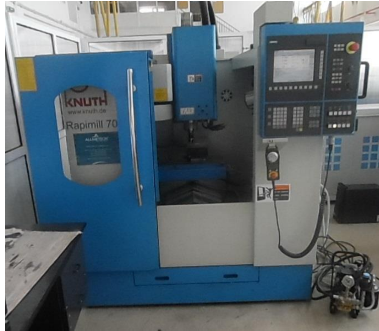
Figure II.2 The milling machine Knuth CNC MILL Rapimill 700.
