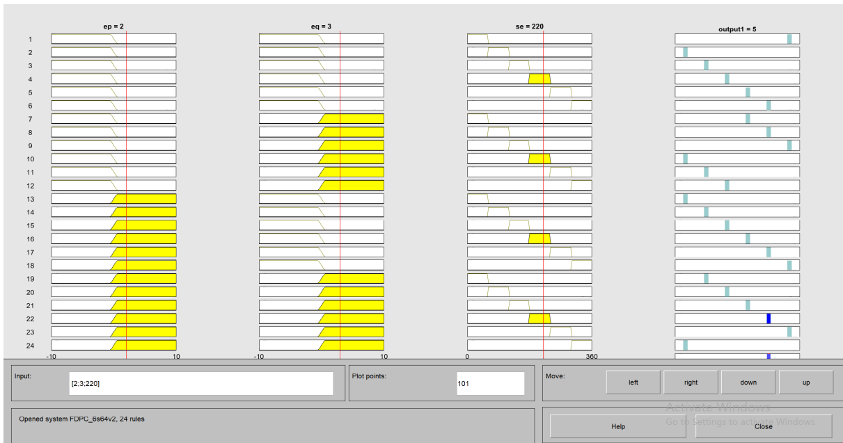
Figure 2.6: Rule Inference DPC 6-sector proposed by Bouafia et al. for [\Delta q, \Delta p, \theta] = [2, 3, 220^\circ] .
