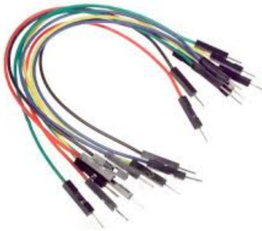
Figure 24: The jumper wires
