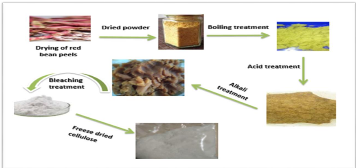
Figure II.3. Diagram showing the steps involved in extracting cellulose from red bean peels.
