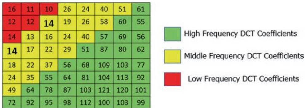
Figure 9 DCT coefficients with size of 8 \times 8
