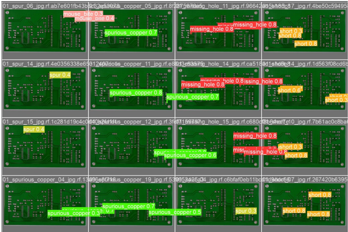
Figure 4.10: Validation Batch Predictions YOLOv8
