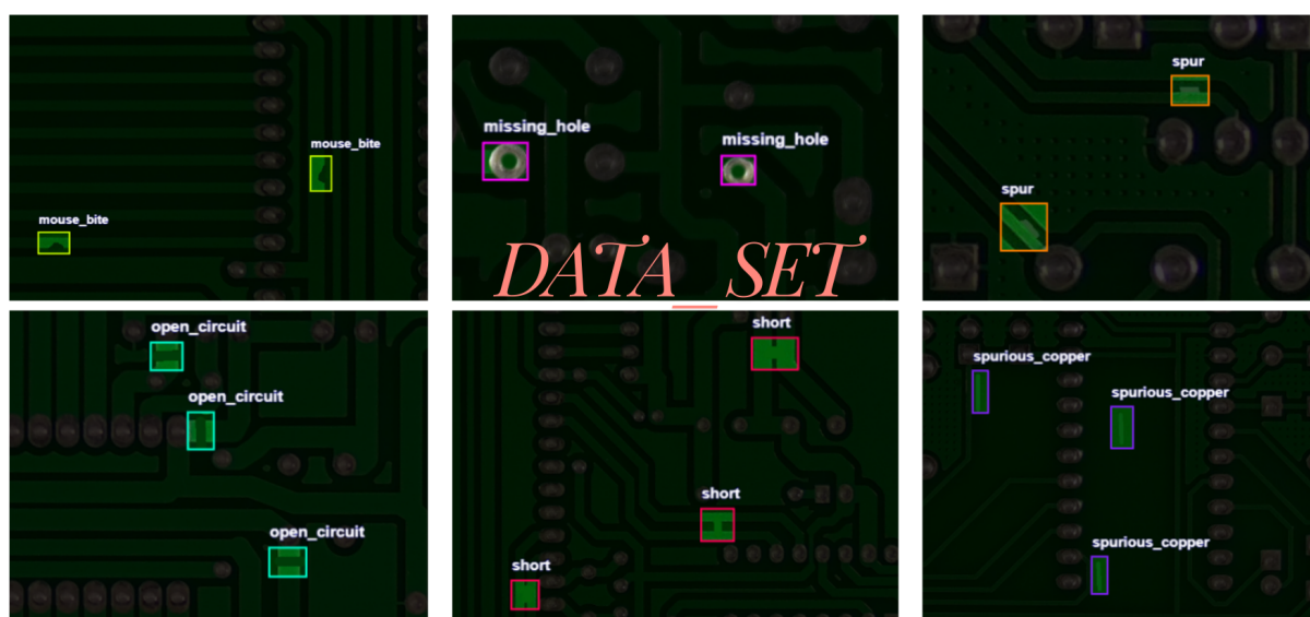
Figure 4.1: Input images with dissimilar defects on PCB: missing hole;spurious copper;open circuit;mouse bite;short;spur.
