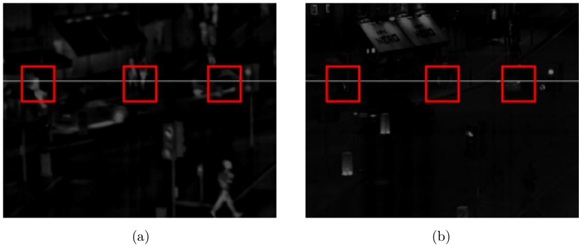
Fig. II.11: The saliency part of infrared image(a) and The saliency part of visible image(b)
