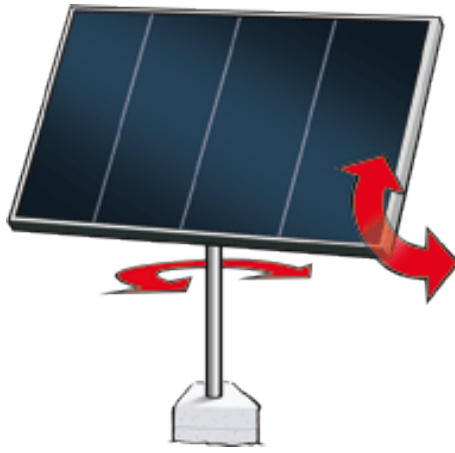
Figure 2.5: Solar panels with Dual Axis Tracking System
