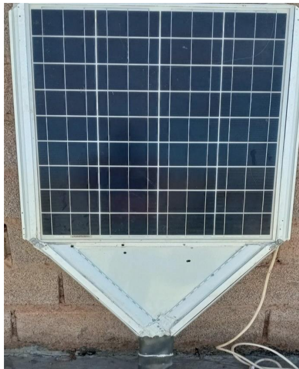
Figure III- 6: The cover and connected photovoltaic panel used in the experimental study.
