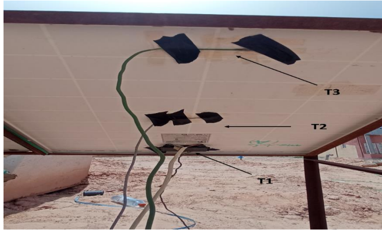
Figure III- 8: Distribution method for K-type thermocouples.
