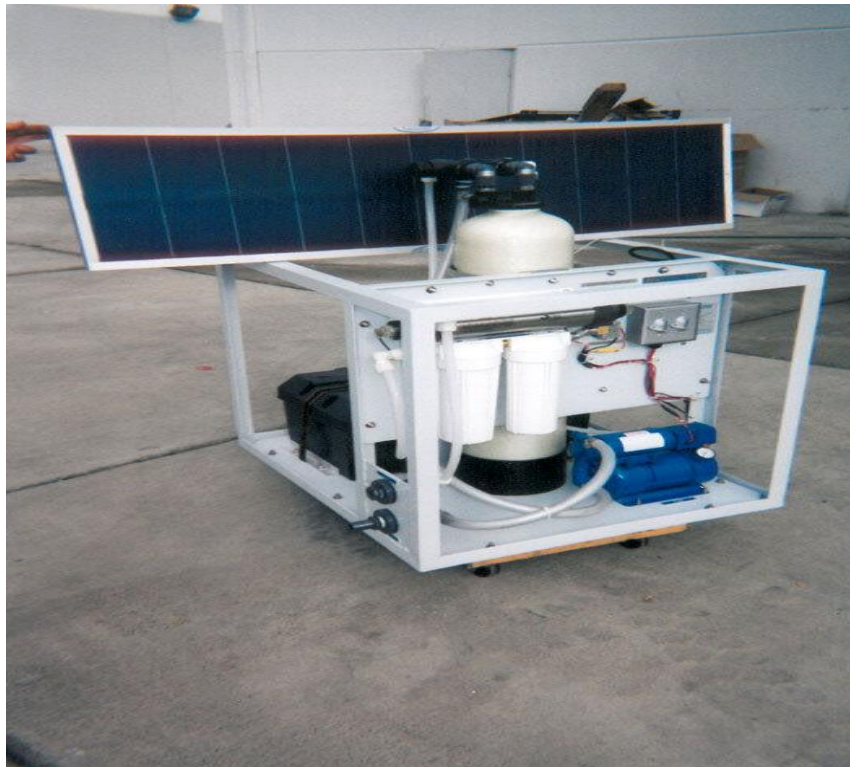
Figure I- 15: Reverse Osmosis Desalination Plant with Photovoltaic Power Source[35].
