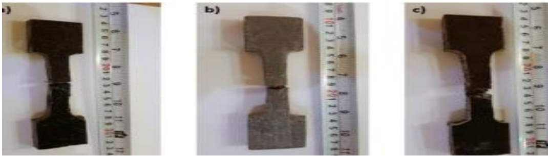
Fig II.8[22]: Failure Modes of some samples of tensile specimens
