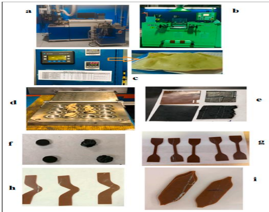
Fig II.2 [14]: (a) Brabender internal mixer. (b) Roller mixer machine.
