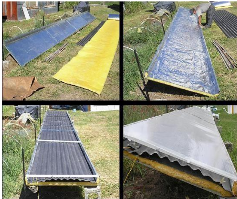
Figure II. 13: Stages in the construction of the collector [24].
