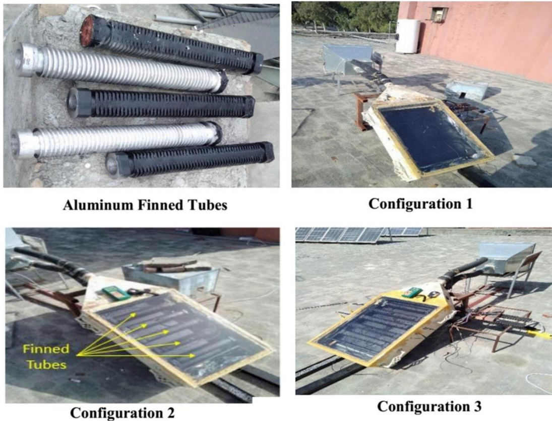
Figure II. 18: Finned tubes and actual experimental configurations[29].
