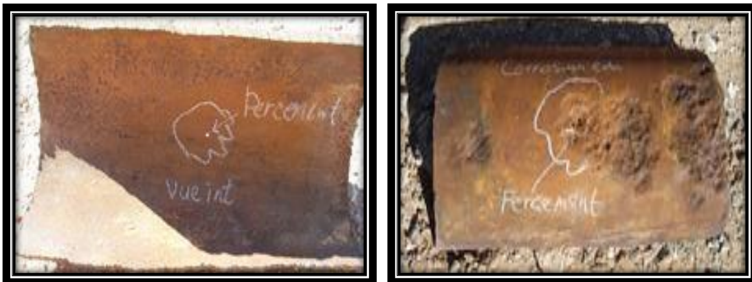
FigureIII.3: External Corrosion of a Buried Pipeline
