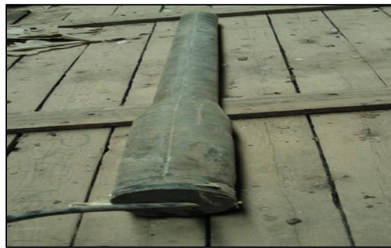
Figure III.11: Ferro-silicon sacrificial anodes. [33]
