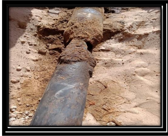
FigureIII.2: Perforation of 4'' Pipe
