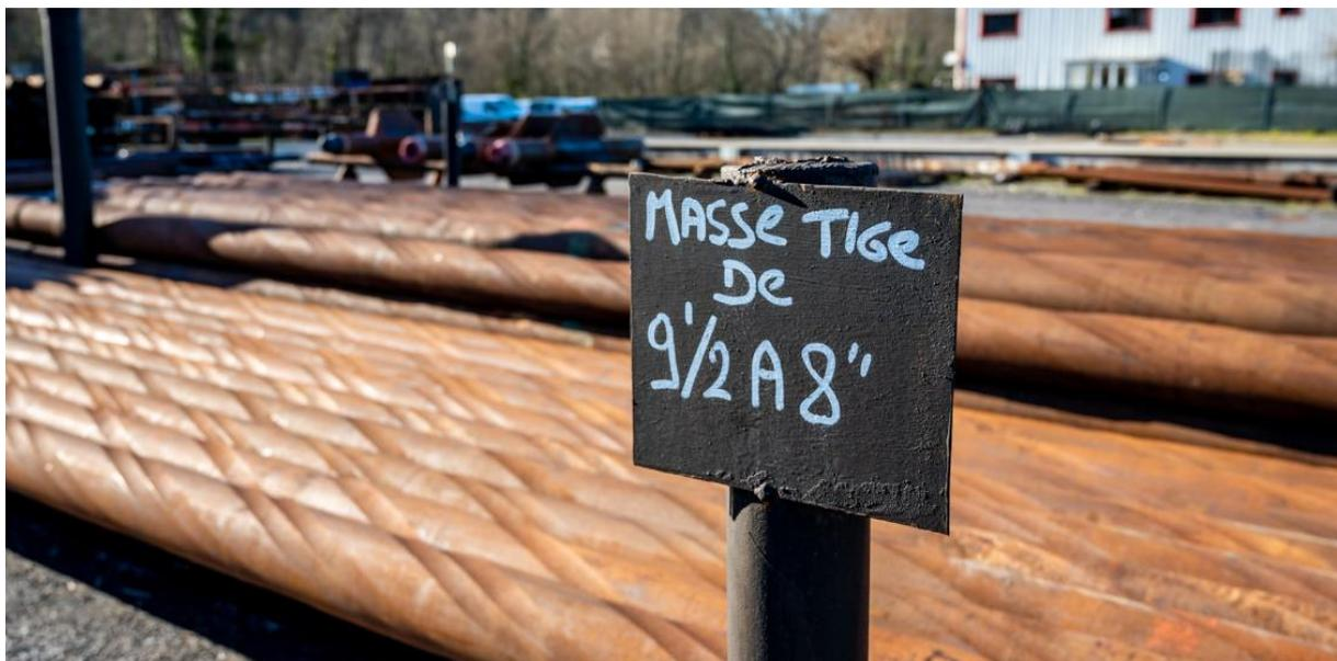
Figure I-15: Les masses tiges [22]
