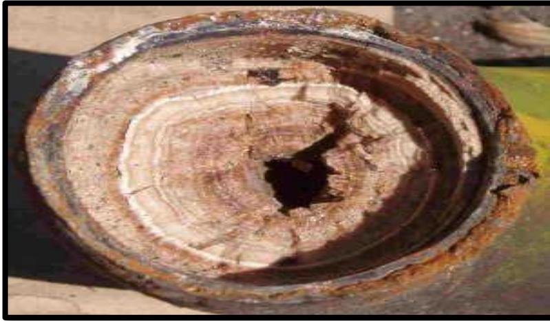
*Figure.II.6. Carbonate de calcium ( $\text{CaCO}_3$ ) [18]*
