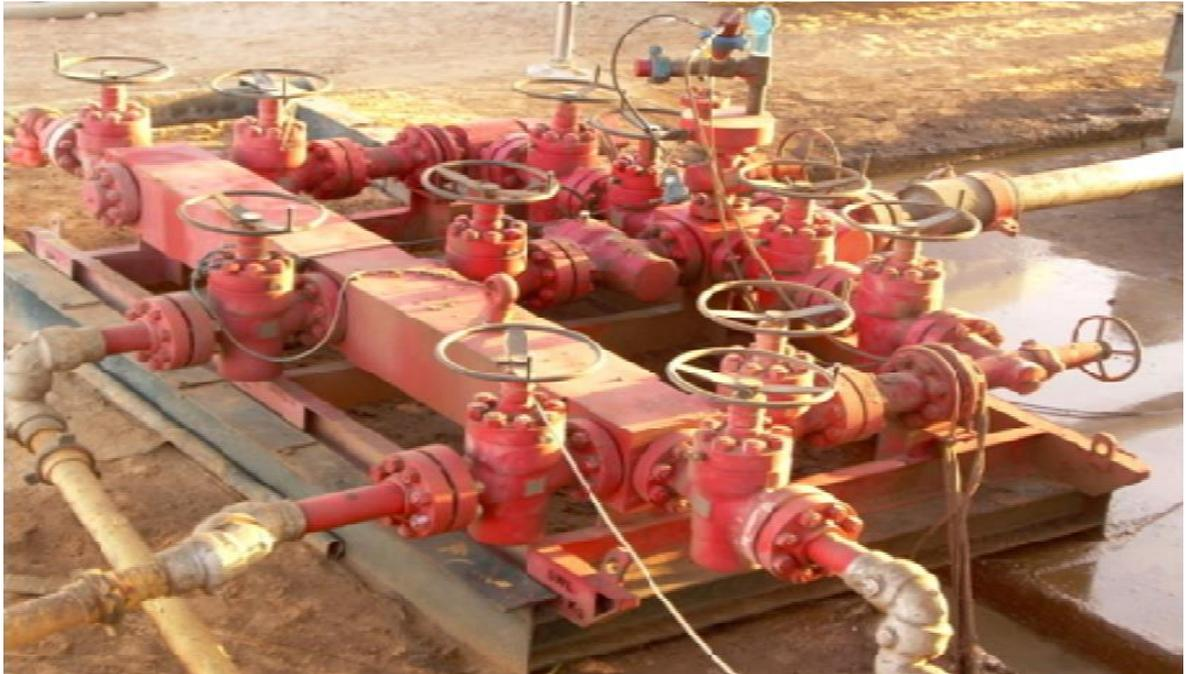
**Figure II.28 : Circuit Choke Manifold [14].**
