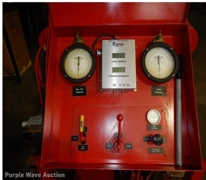
Figure II.30 : Choke Panel [14].
