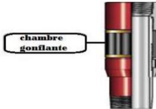
Figure I.13: liner top packer.
