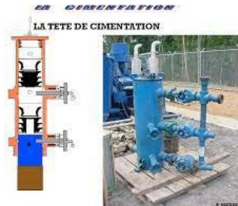
Figure II.1: La tête de cimentation.
