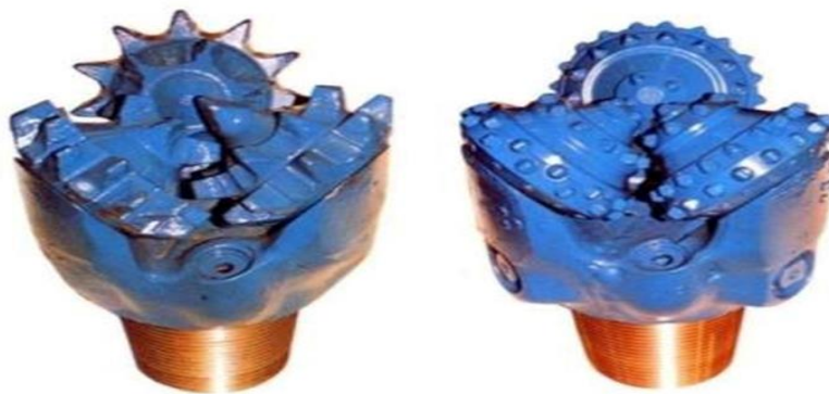
Figure 01: Milled tooth bit and Tungsten Carbide Inserts bit[3] .
