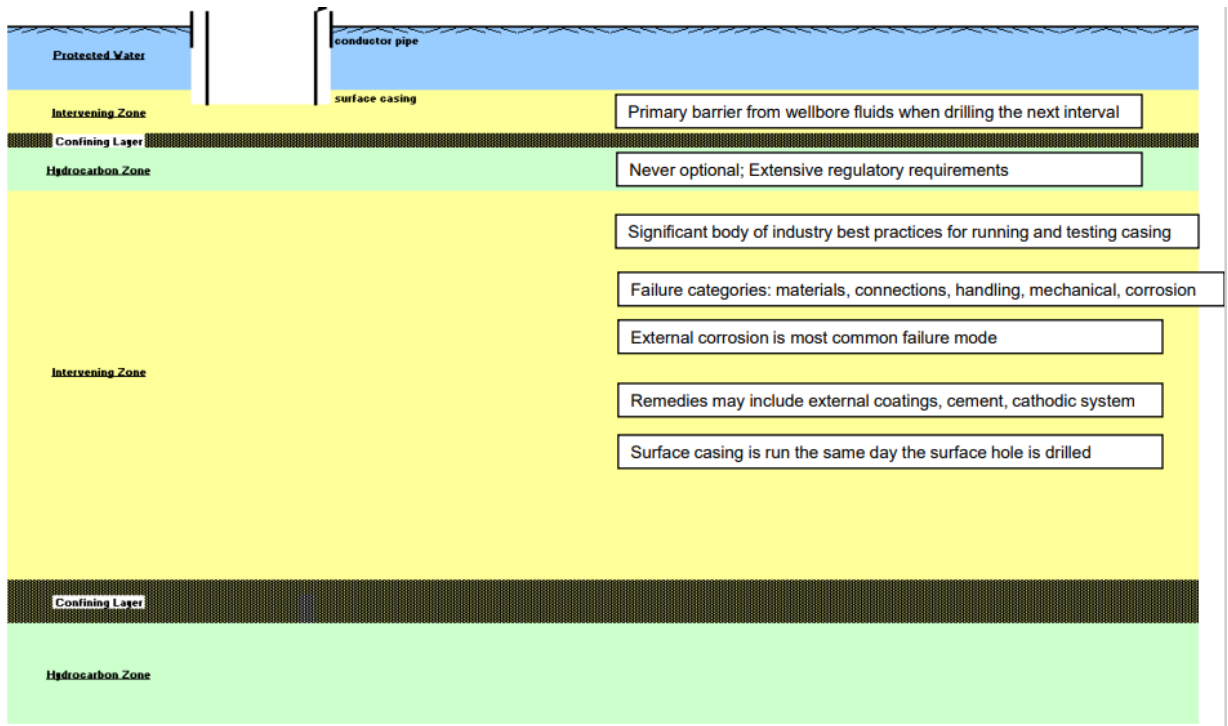
Figure 28: Place the surface casing in place.
