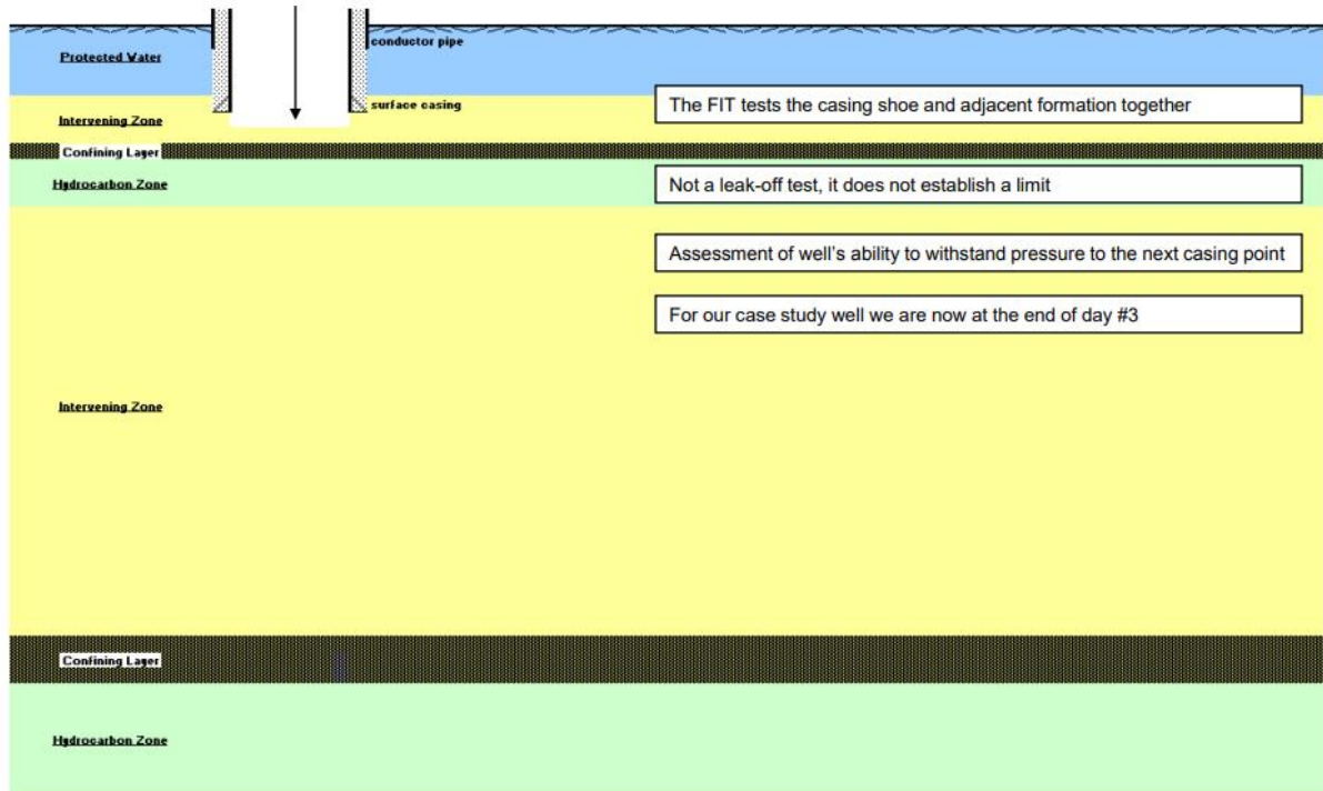
Figure 30: Testing of surface casing shoe.
