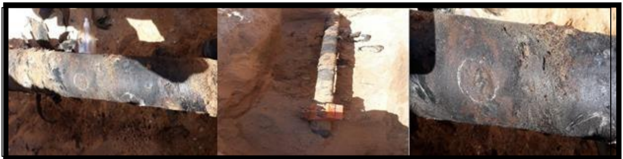
Figure II-6 : Perforation Level of 4" Pipe
