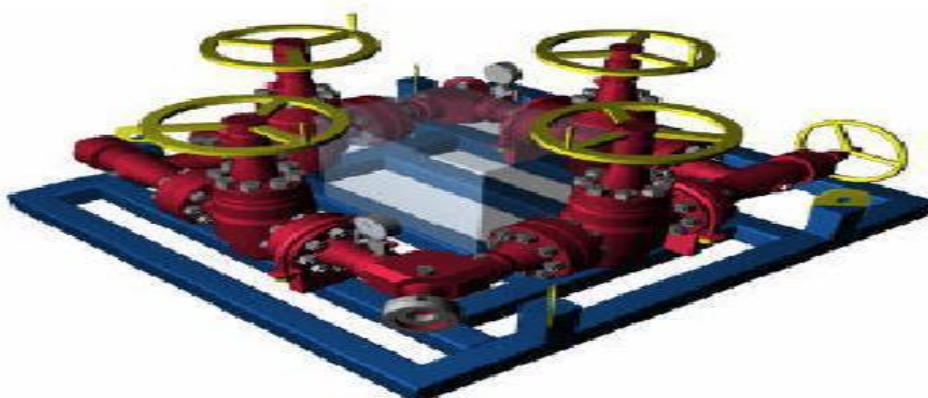
Figure.III.29. The choke manifold[8]
