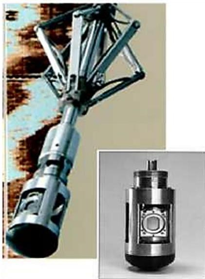
**Fig.15:** Outie UBI "Ultrasonic Borehole Imaging"
