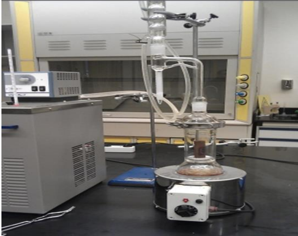
Figure 27: An image illustrating a water saturation measurement device (Soxhlet) [16].
