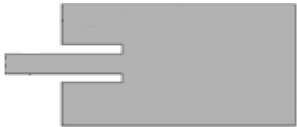
Figure I.10: Patch antenna with slots
