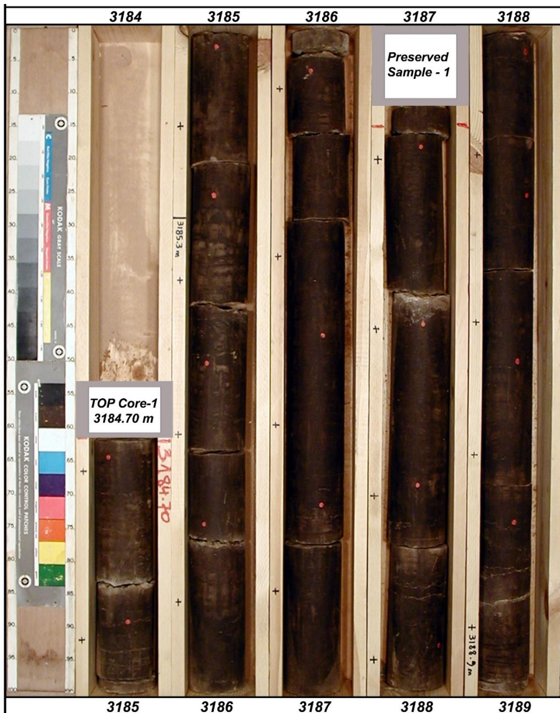
Fig. 27: Core #1 taken during drilling of well GS-38
