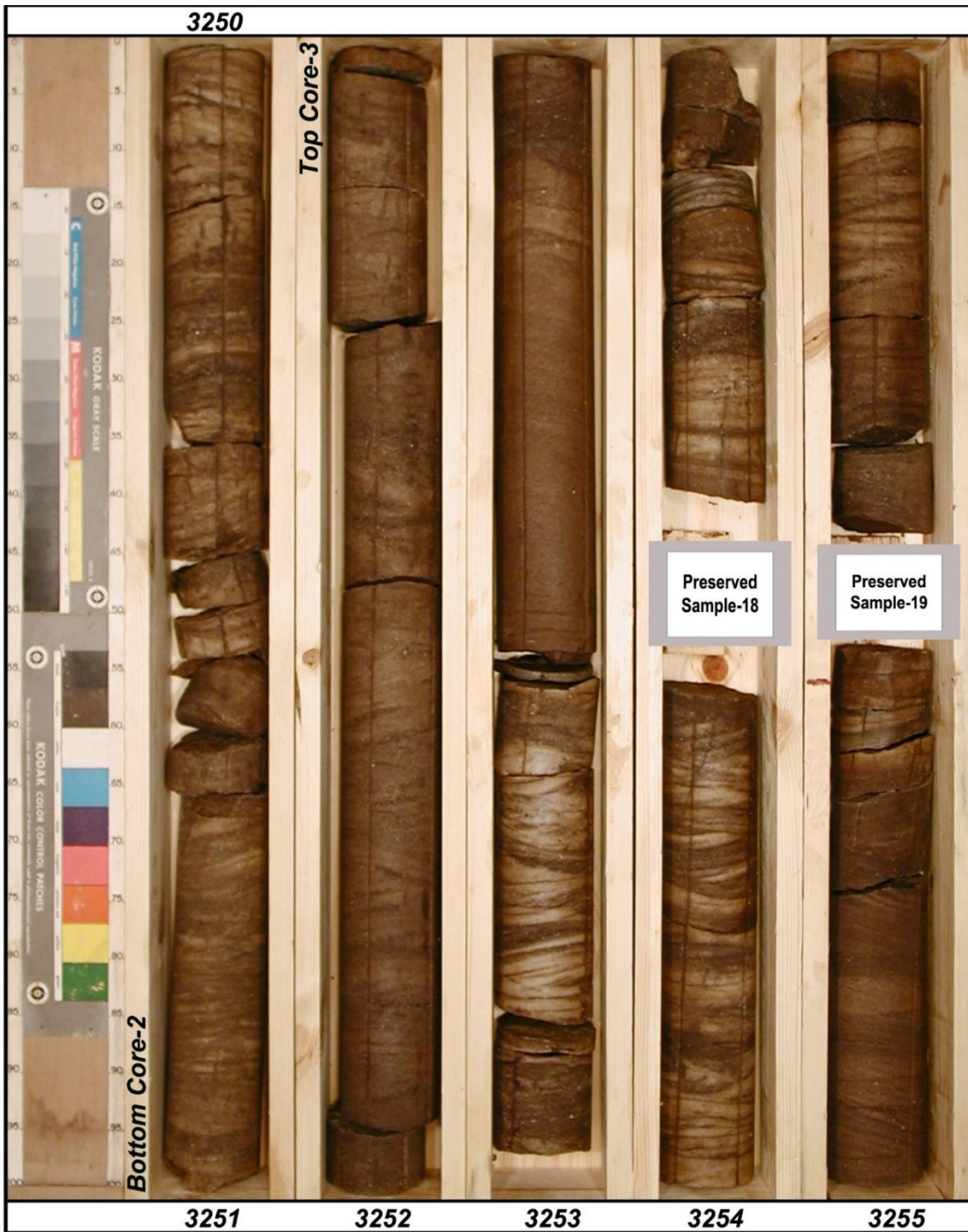
Fig. 25:Core #2 taken during drilling of well GS-36
