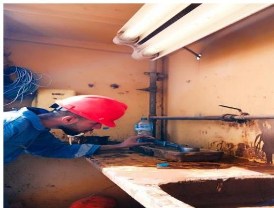
Figure 17 Mud Balance Calibration
