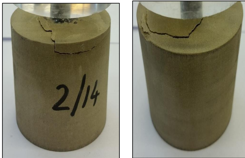
Figure III.18. Comportement à la rupture (Brine, Sample 2-14)
