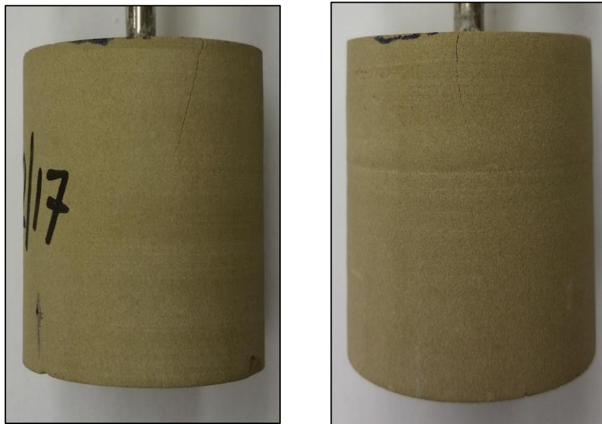
Figure III.16 Comportement à la rupture (Brine, Sample 2-17)
