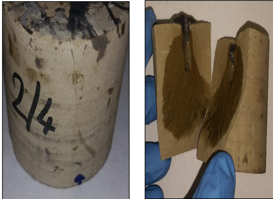
Figure III.22 Comportement à la rupture (25 ppt Linear Gel, Sample 2-4)
