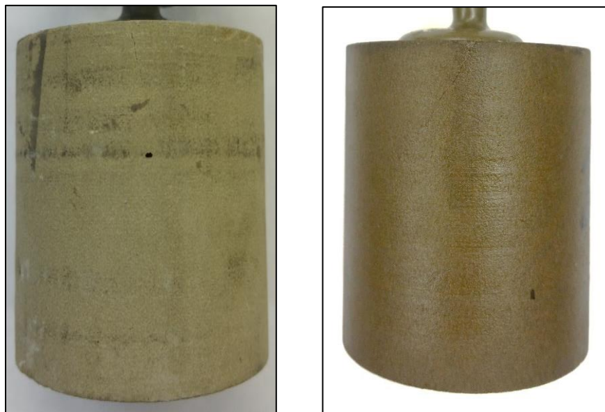
Figure III.11. Comportement à la rupture (25 ppt Linear Gel, Oil Saturated Sample 2-15)
