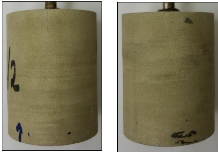
Figure III.30 Comportement à la rupture (40 ppt Linear Gel, Sample 2-2)
