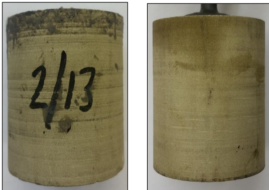
Figure III.42 Comportement à la rupture (40 ppt Crosslinked Gel, Sample 2-13)
