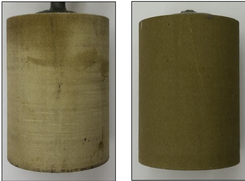
Figure III..9. Comportement à la rupture (25 ppt Linear Gel, Brine Saturated Sample 2-12)
