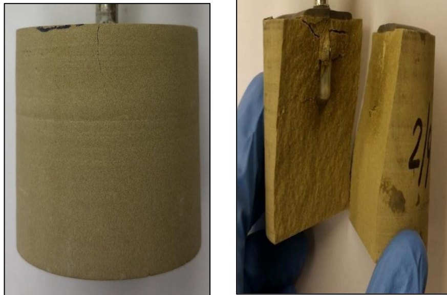
Figure III.40 Comportement à la rupture (40 ppt Crosslinked Gel, Sample 2-9)
