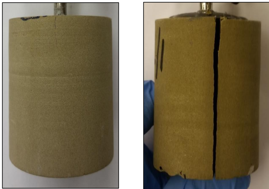
Figure III.36 Comportement à la rupture (25 ppt Crosslinked Gel, Sample 2-1) .
