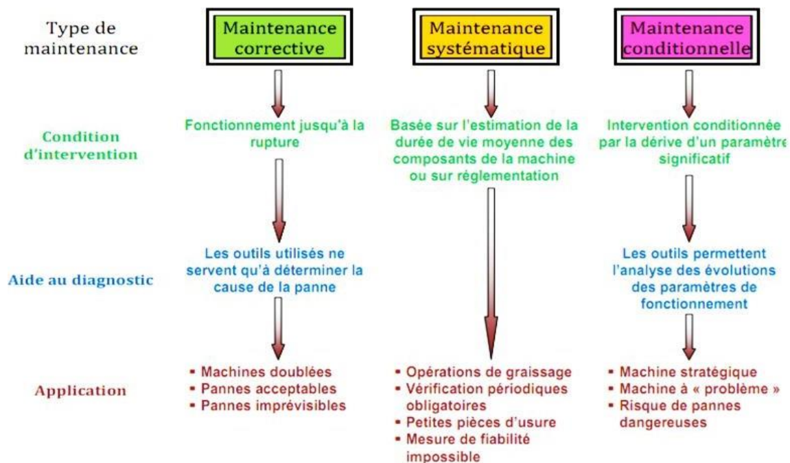
Figure I.2: les types de maintenance
