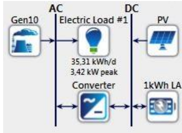
Figure III. 1: electrical assembly of the hybrid system
